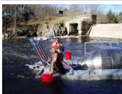
Researchers removing very young salmon bound for the Atlantic from water-powered traps in a river.
