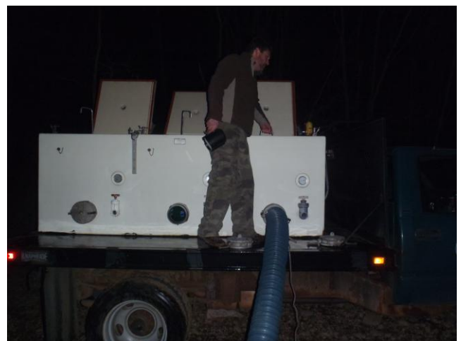
Once the hose is connected, Tim Wildman raises the knife gate to release the water and fish for a 20 ft descent to the river.
