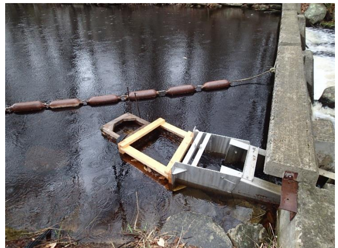
Lower Guilford Lake Fishway- Fish need to climb one section of steppass fishway at the top to get over the low dam. This year, we installed our 'roving fish counter' to get a one year snapshot of how many alewives use this fishway. Later next month, a UMass research team will sample the lake for young alewives to correlate those numbers to the numbers of adults counted passing through this fishway.
