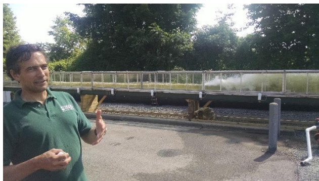
Dr. Ted Castro-Santos of the Conte Lab explains the Burst Speed Test Flume in the background. At the time, lots of water was racing down the flume and the upper part (to the left) was at what is referred to as super-critical flow. The lower part was sub-critical flow and you can see the turbulent hydraulic jump in the middle. Such a 'jump' often occurs below dams where water is coming off a spillway.
