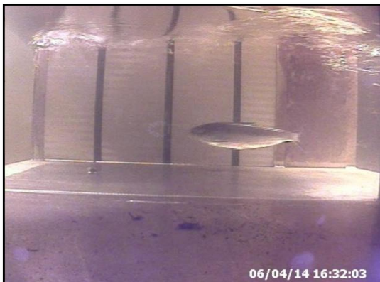
A Blueback Herring cranks through the video gallery of the Moulson Pond Fishway. You can see the retro-reflective background behind the fish that I suspect is causing problems with the infrared camera. The black vertical lines are 6" apart.
