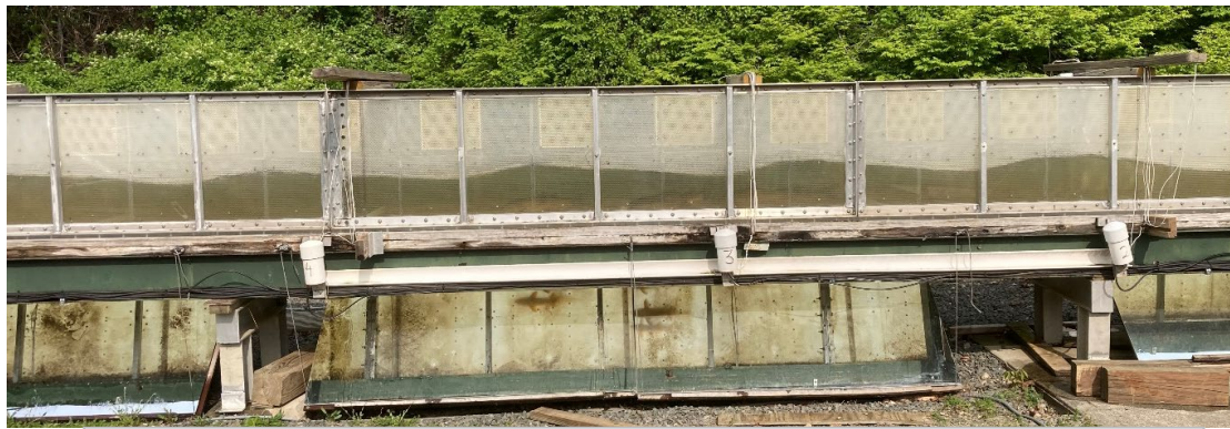
Aquatic Biomechanics and Kinematics Station (ABiKiS), developed by Ted Castro-Santos (USGS Conte Lab) to test and describe fish swimming abilities, a much understudied area of management importance for fish passage. Two white suckers are shown and monitored by PIT tags and high speed video.
